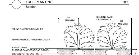
During Excavation/Bed Preparation if Extreme Conditions are Encountered (Water, Rock, Gravel...) Notify GJA INC Immediately.
