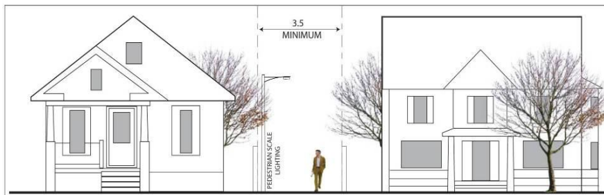
Figure: Design guideline for residential mid-block connection. The walkway should be at least 3.5m wide and include pedestrian-scaled lighting.
