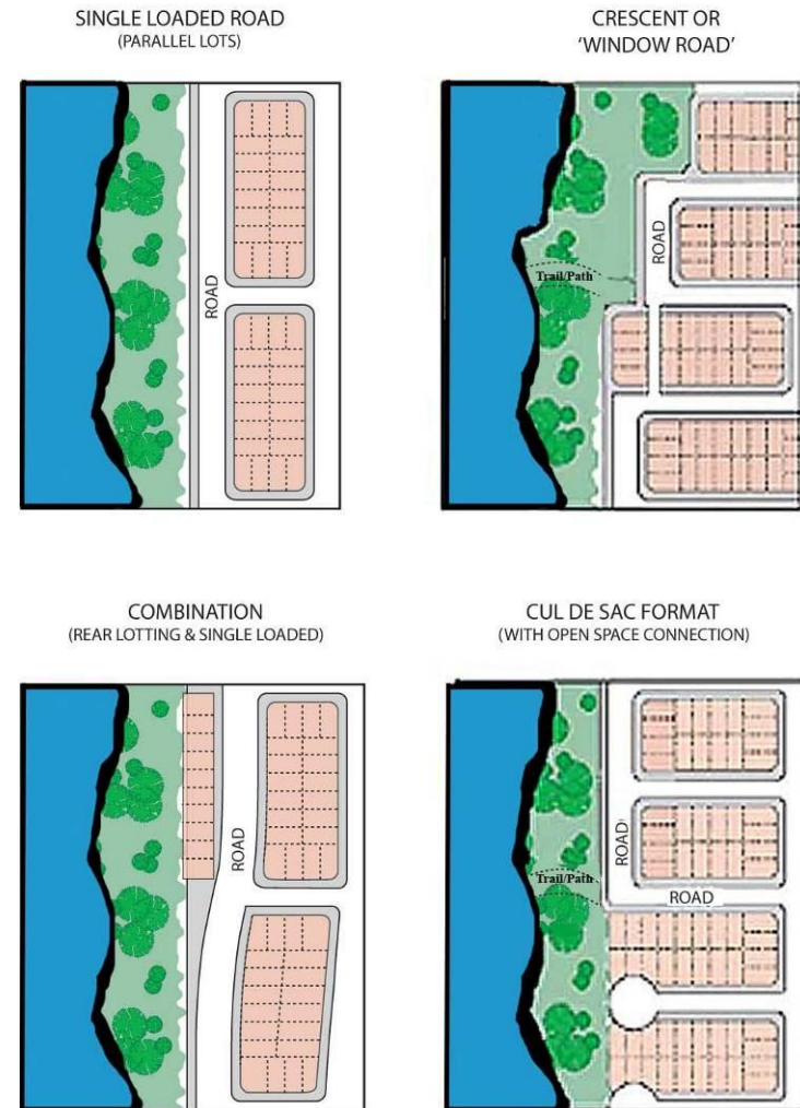
Figure: Guideline for block and open space interface options. A positive interface should be achieved with open space wherever possible. Rear lotting should be avoided wherever possible.
