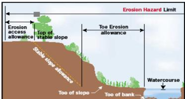
The toe erosion allowance is the setback that ensures safety if the toe of the slope adjacent to the watercourse erodes and weakens the bank, thereby increasing the risk of slope failure.
