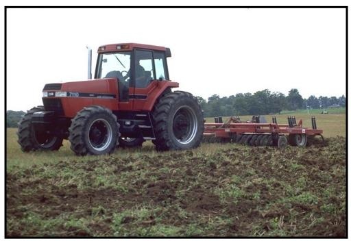
(Figure #3) Incorporation of biosolids with an offset disc
